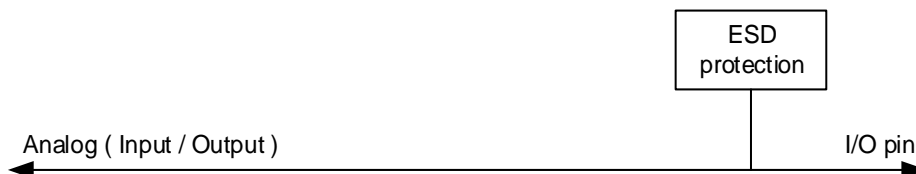
Figure 10-4. Basic structure of Analog configuration
